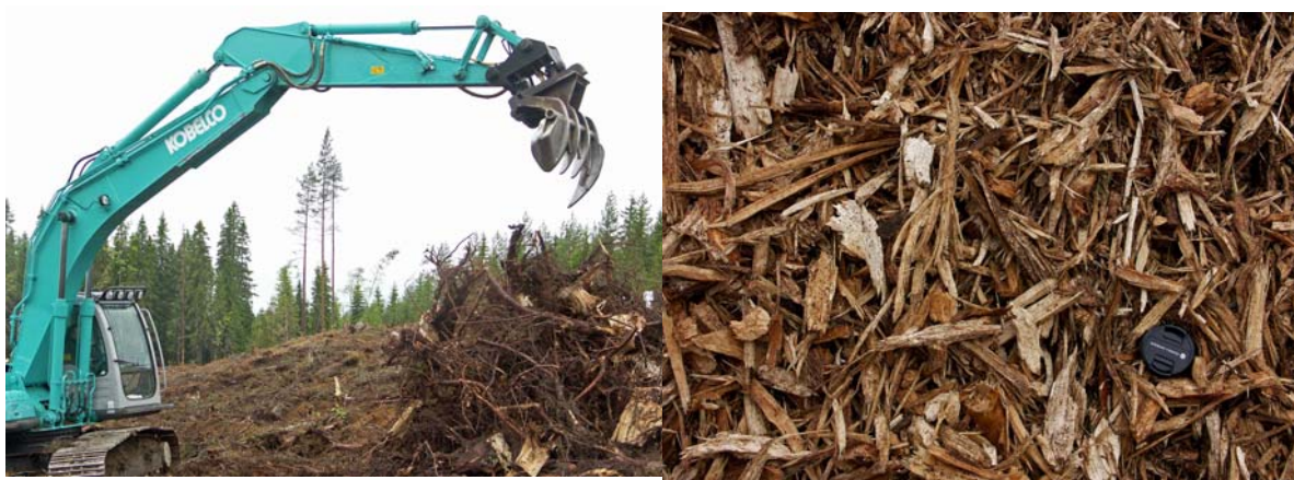
Figure 15. Extraction of stumps from final felling areas and hog fuel produced from stumps.
