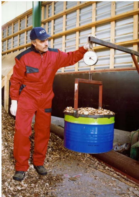
Figure 6. Measurement of bulk density in small-sized heating plant in Finland.
