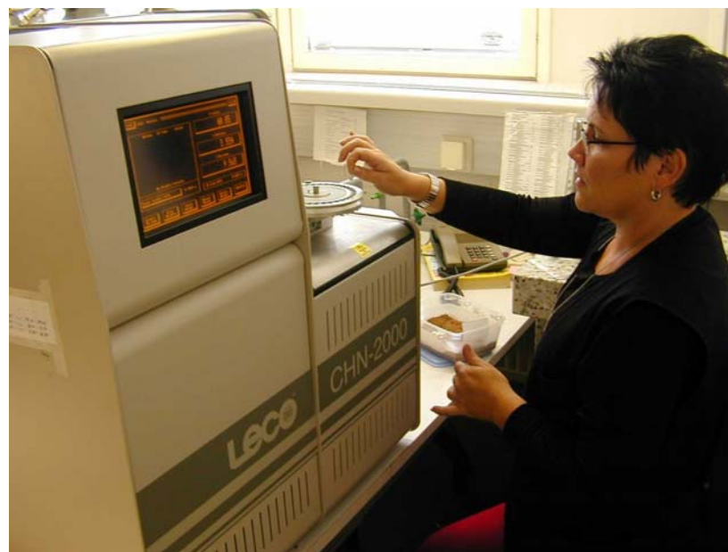
Figure 5. Analysis of carbon, hydrogen and nitrogen by CHN-analysator.
