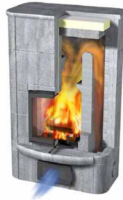
Heating principle of a heat-retaining stove (Courtesy of Nunna Uuni Oy)
